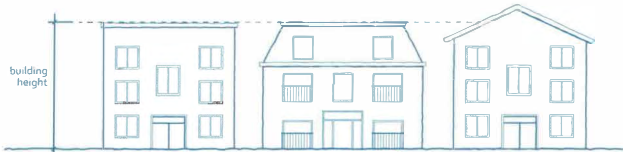
Figure 21-7: Building Height Measurement
