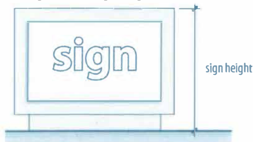
Figure 15-7: Sign Height Measurement
